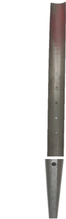
1 Bypass wedge showing wedge ends (chisel and blunt), middle, and rod end
