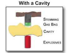
Block a void or cavity that the drilled hole has penetrated. Plug exploration holes.
