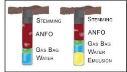
If your holes have only a few feet of water, try dropping a Gas Bag on the water to seal off the hole. Add a little stemming and use ANFO instead of waterproof explosives. Generally you can use this system up to 6 times the borehole diameter of water.
