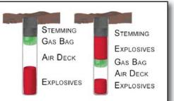
Save 15% to 35% of the total explosive load and still have excellent dig-ability. It's possible to reduce vibration and noise in addition to cost savings.
