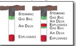
Hole spacing should be 15 to 24 times the borehole diameter in inches depending on the local geology. If the hole is over 50 feet deep, two or more charges should be used for better explosive distribution. Usually about 60% of the total charge should be in the bottom. Charge weights should range between 3% to 10% of the total charge in a normal production hole.
