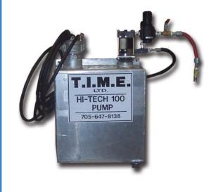
The Haskel pump is used where high psi output is required. The air drive of the pump requires a minimum pressure of 25 psi (1.72 bar) to actuate the air cycling valve spool. However, 40 psi is the recommended minimum for long term reliable operation. Maximum air drive pressure is 125 psi (8.6 bar).
