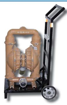
This cart was custom designed for a customer that needed to move the three inch Nomad pump NT80 with a weight of 100 lbs from one location to another.
