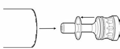
**K**, Remove Inner Cylinder (8) from Wear Sleeve (10).
