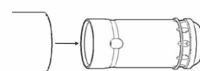
**L**, Remove Piston (11) from Wear Sleeve (10).
