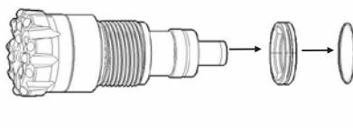
**E**, Remove Chuck (14) from Drill Bit (15).
