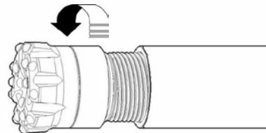
**D**, Remove Bit Retaining Ring (13) from Drill bit (15). Remove 'O' Ring (12) from Bit Retaining Ring (13).
