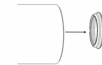
**J**, Remove Air Distributor (7) from Wear Sleeve (10). Remove 'O' Ring (6) from Air Distributor (7).
