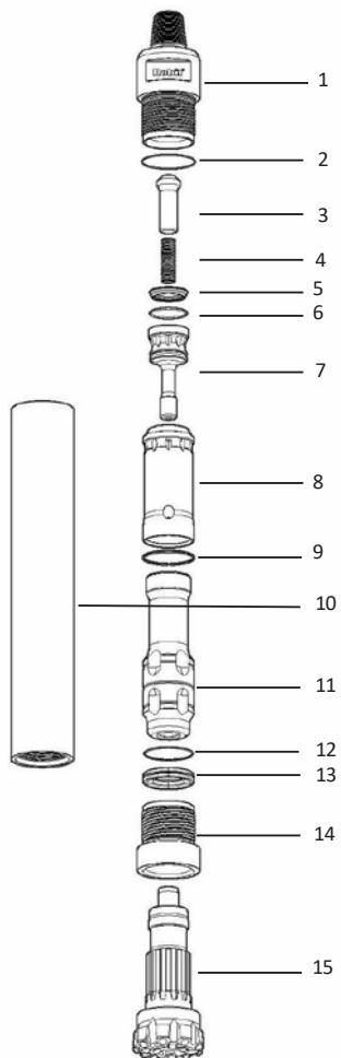
**A**, When dismantling hammers it is essential that the wear sleeve is clamped in the correct position.
